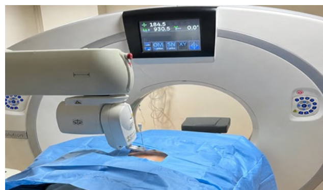
Figure 3: Clinical setup showing MAXIO robotic alignment with the planned trajectory during a biopsy procedure.
